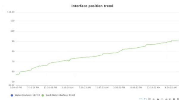
Picture 2: Illustration of the process situation where the sand is steadily accumulating.
