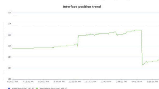
Picture 3: Illustration of a process situation where sand removal is executed.
